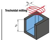
$\begin{array}{l} a_{\text{p}} = \text{max. 3xD} \\ a_{\text{e}} = \text{depending on the workpiece} \\ \text{material} \end{array}$
