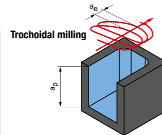
a<sub>p</sub> = depending on max. machining depth of the tool
