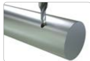
Eccentric holes on convex surfaces.
