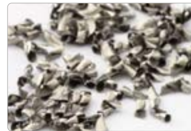
Compact, short and curved chips are easily evacuated and guarantee a long tool life as well as high process reliability.
