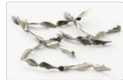
Long chips cause chip jamming and difficult evacuation. This leads to overheating with consequent build up edges. The result is a cutting edge breakout in short time.
