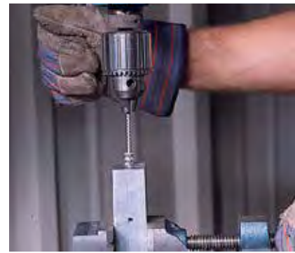
Crosshole deburring an aluminum manifold.
