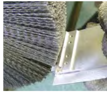
Removing burrs from an aluminum heat sink.
