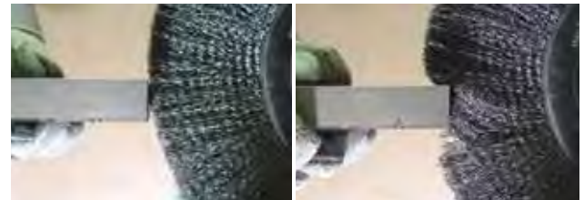
Correct Wire Tips Doing the Work
