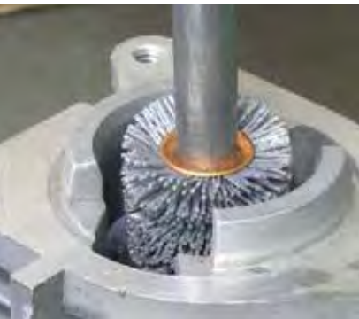
Deburring internal bores of a cylinder head.
