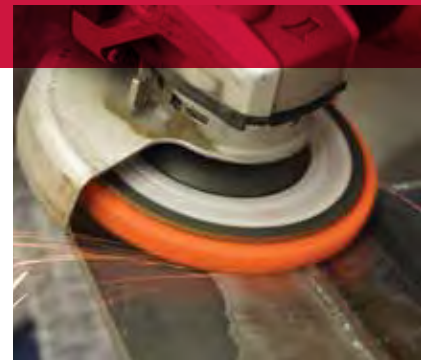
Weld cleaning with a strip disc.
