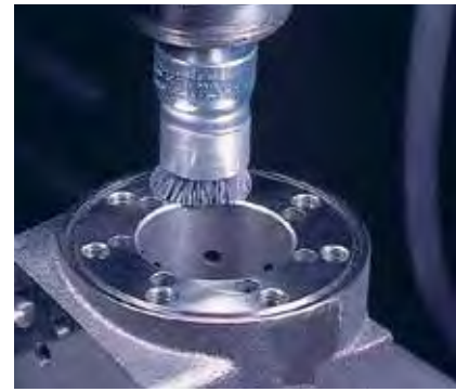
Blending tool marks on a hydraulic component.
