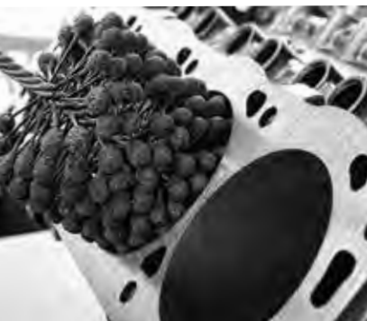
Engine cylinder head honing.
