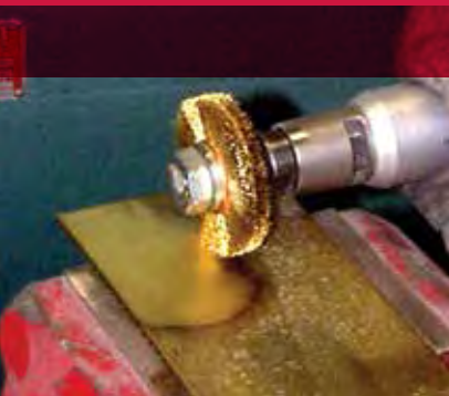
Creating an antique finish on a brass plate.
