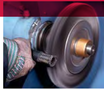
Removing rubber coating from a hydraulic hose.
