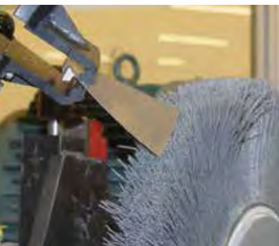
Deburring the tip of a turbine blade.
