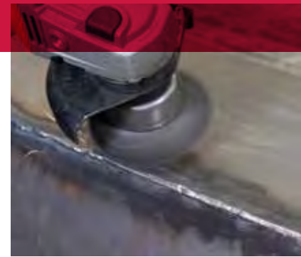
Knot wire cup brush removing heat discoloration.
