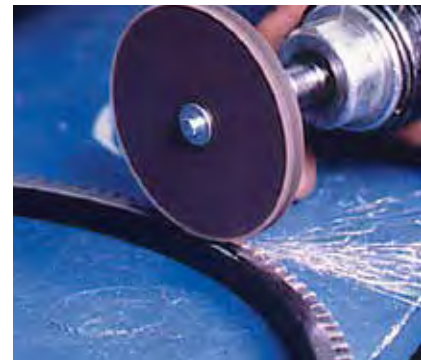
A unitized wheel deburring a ring gear.
