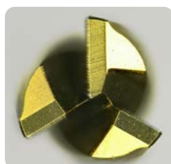
Edge wear after 20 m in CoCr alloy
