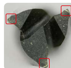
Edge wear after 7 m in CoCr alloy
