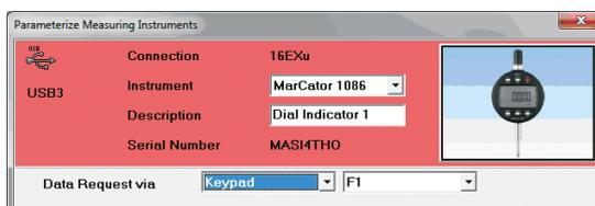
Via a “*MC-I Switch*” (foot switch). Here you can select additional values with either “*per Measurement*” (i.e. each time the switch is operated a value will be sent) or “*with Measurement No.*” (i.e. the values that are to be send to the measuring cycle after X-times activation of the switch).
