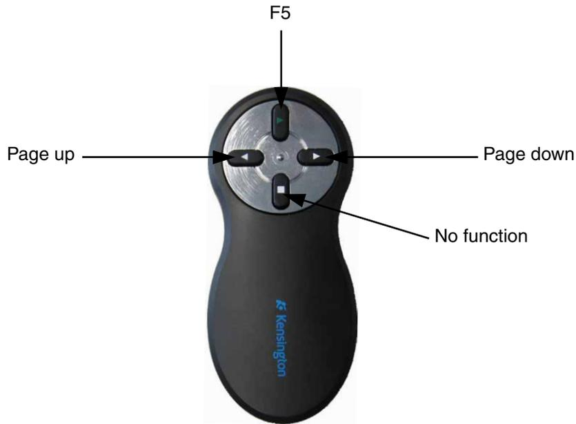
The Remote Control (4102221) no external driver is required. Once a USB receiver has been connected Windows own driver will be installed. After the this driver has been installed you can press a button on the remote control which simulates a keyboard command, see above illustration. With MarCom these keyboard commands can be assigned functions.
