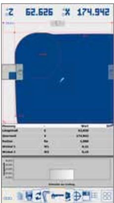
Determine up to 5 measurement results (Z, X, radius, angle 1, angle 2)
