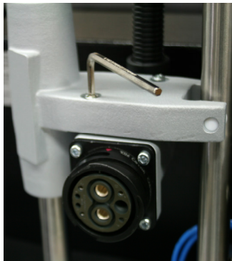
Fig. 9 Securing the connector unit
