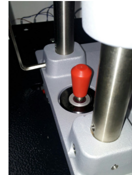
Fig. 6 Inserting the guide unit in the machine
