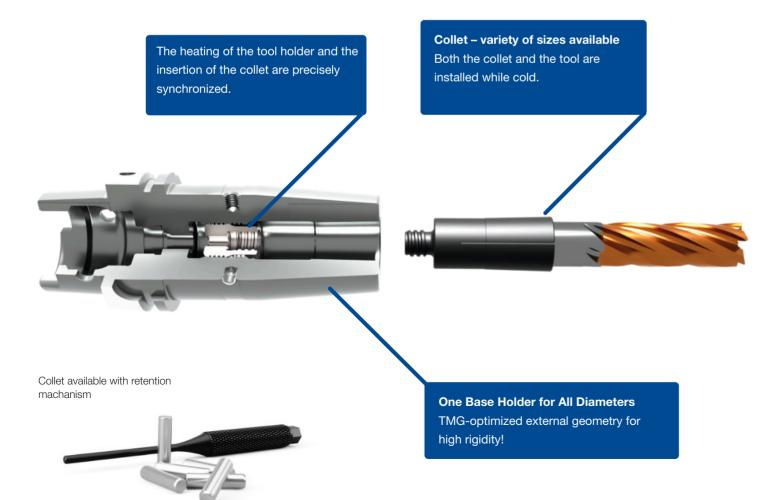
The new Bilz TMG clamping system combines the strength of shrink chuck technology with the flexibility of collet solutions. The system consists of base holder and specially coated collets. Cutter shanks (HSS) from 3 to 32 mm can be clamped with unprecedented clamping forces—for example, over 950 Nm for a Ø20 mm tool shank when automated with our ISG 3460 shrink machine, the latest and most advanced model available.
