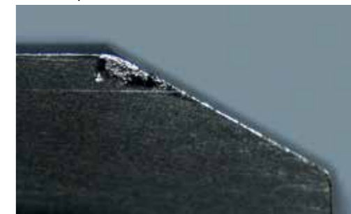
HSS reamer DIN 212 after 250 bores
