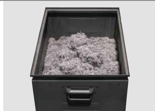
Comparative chip volume: The chip volume is considerably reduced depending on the chip shape and material. In the case of cast iron chips, a reduction in volume of approx. 1:5 is possible and with long turned chips from steel, a reduction of approx. 1:50 is possible.
