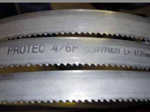
Saw blade with lateral scoring
