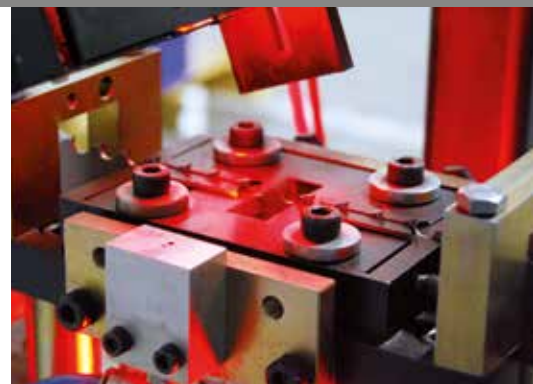
Online process control during saw blade manufacture
