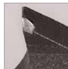
Damaged tooth, not run-in
