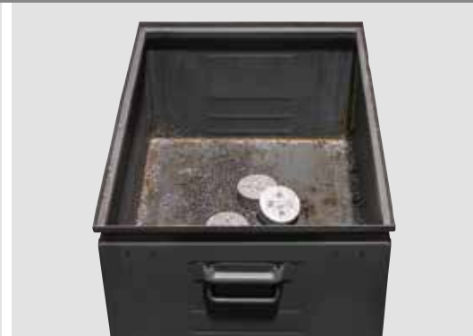
Comparative chip volume: The chip volume is considerably reduced depending on the chip shape and material. In the case of cast iron chips, a reduction in volume of approx. 1:5 is possible and with long turned chips from steel, a reduction of approx. 1:50 is possible.
