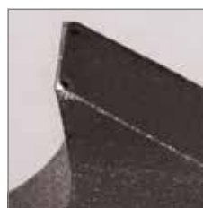
Damaged tooth, after running-in
