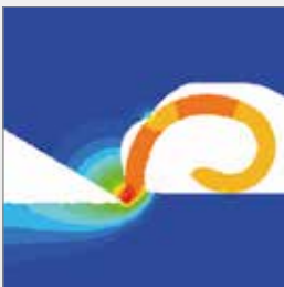
New tooth design with chip breaker
