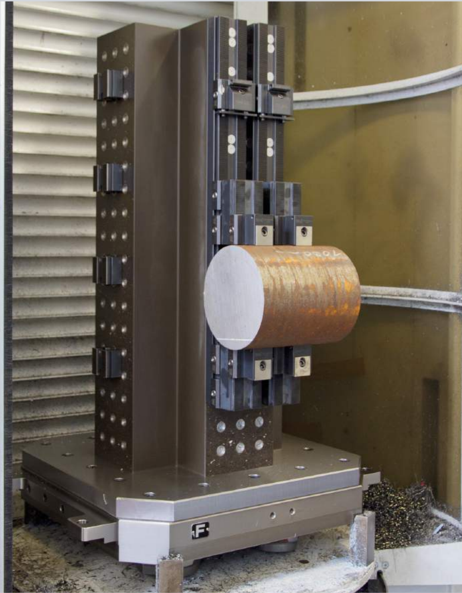
Round blank Ø 350 mm clamped with Power Clamp modules and riser base rails.
