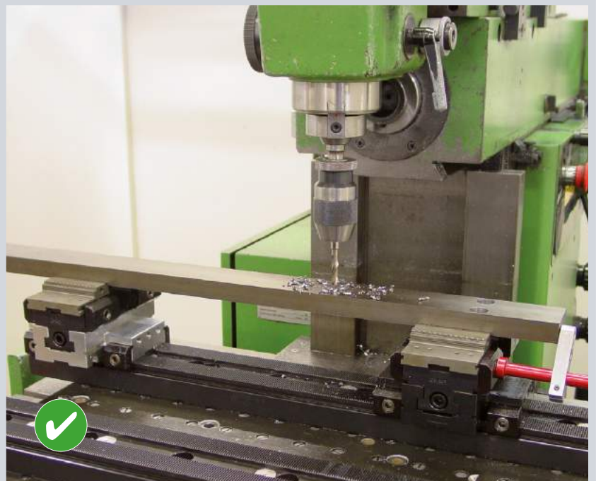
Surface milling making two faces parallel... ... after drilling a steel bar the self centric vises can moved sideways in 2mm steps.
