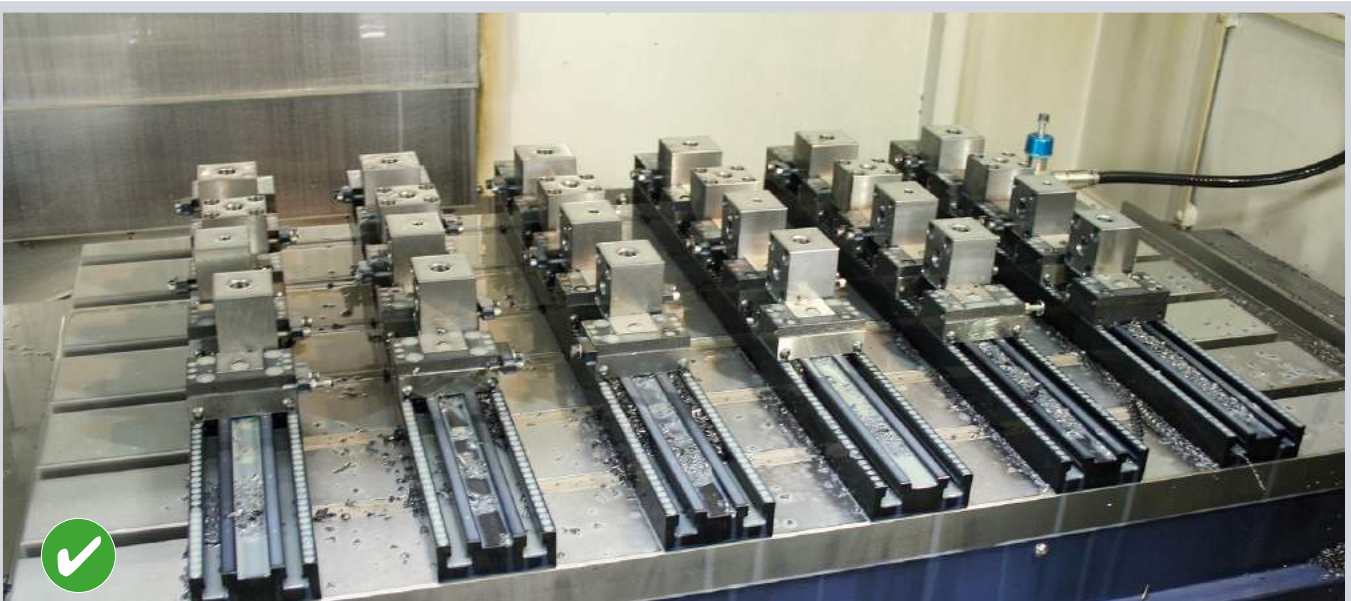
Not bad used but probably he would make even more parts maybe there were no more clamp modules available? This is the older Compact Clamp in operation.
