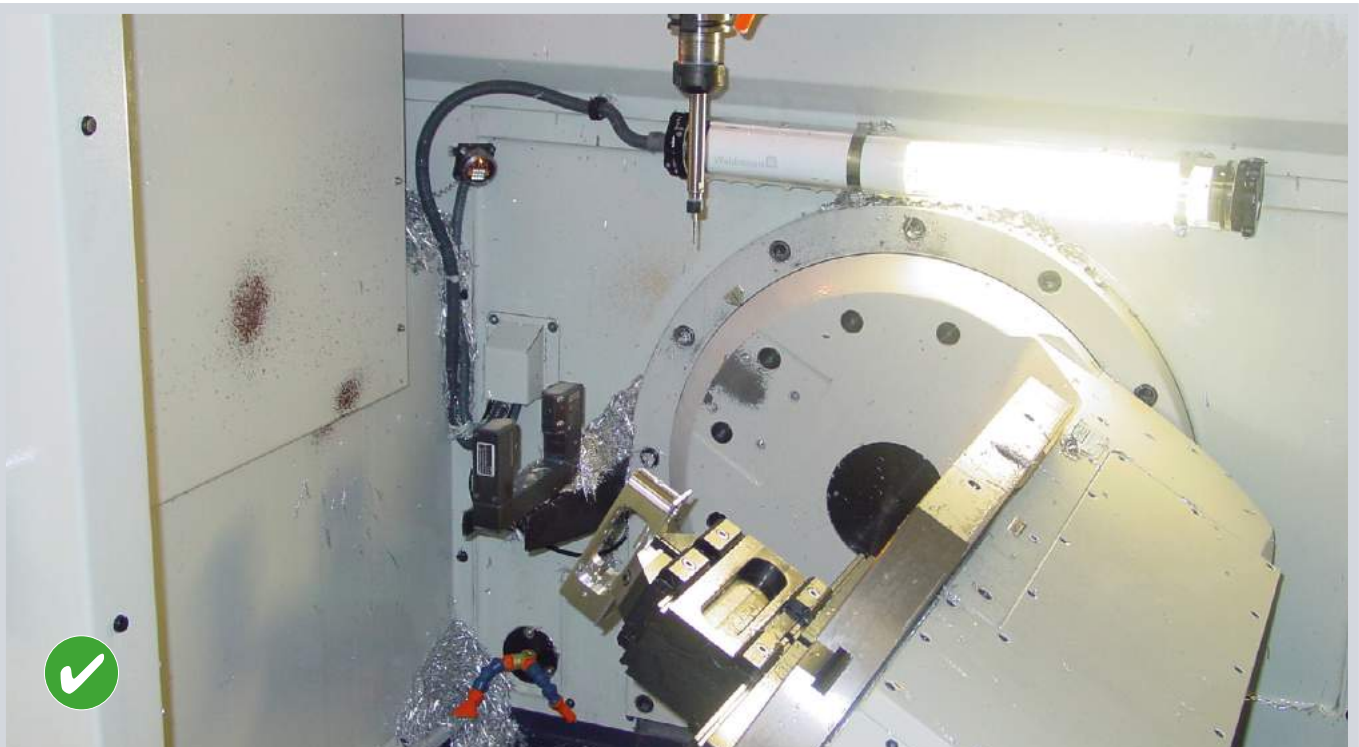
5 face machining with good access to the workpiece.
