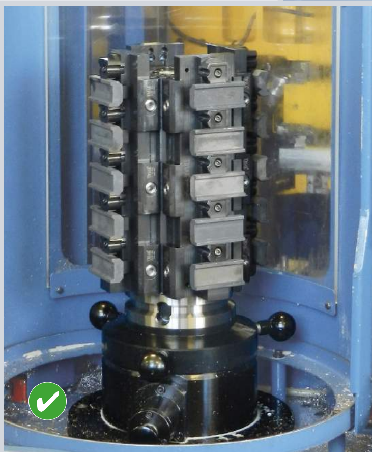
Multiple workholding in high density on 5-axis machine with micro clamp modules.
