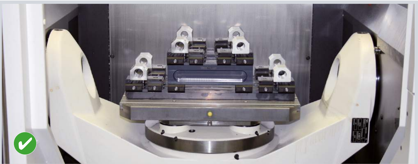
8 parts all machined on 3 faces.
