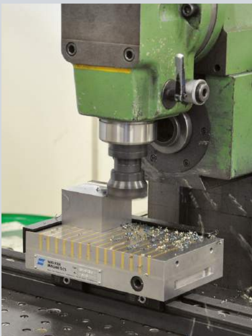
Surface milling making two faces parallel... ... after drilling a steel bar the self centric vises can moved sideways in 2mm steps.
