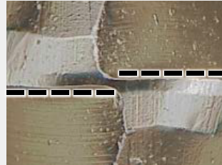
Conventional profile after 10 minutes of use
