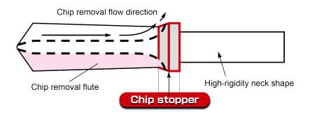
Chip-removal stopper technology and highrigidity neck shape enables high-accuracy drilling of minute holes.
