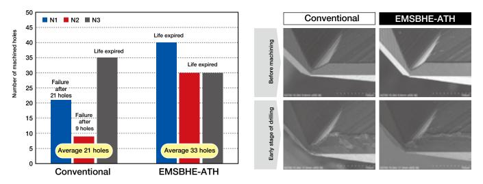
EMSBHE consistently reaches end of life without breakage. Improved machining stability with 60HRC class high hardness steel.
