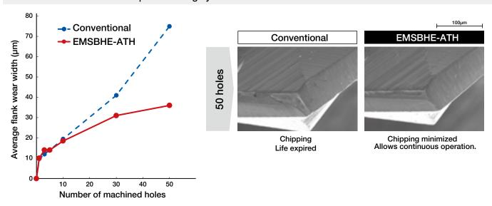
Flank wear reduced to less than half that of conventional tools. Allows continuous cutting-estimated life of at least 100 holes.
